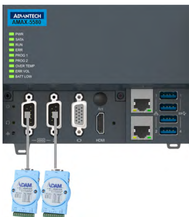
Figure 3.4 ADAM-4520 Isolated RS-232 to RS-422/485 Converter installation example
