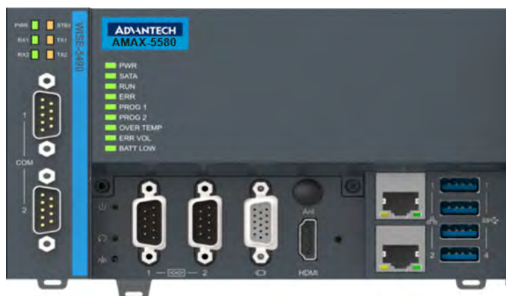
Figure 3.3 AMAX-5490 Serial Expansion module installation example
